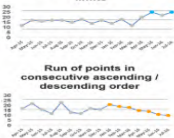
Two out of three points close to the process limits
